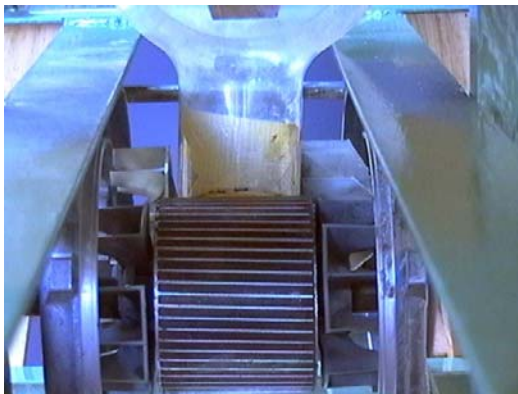
Fig. 5: The funnel is best sealed with duct tape.
